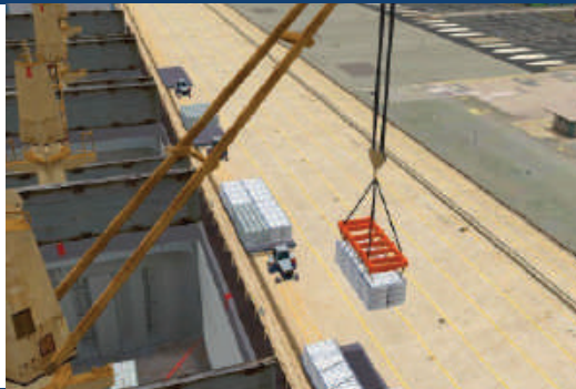
Ship Pedestal Crane
